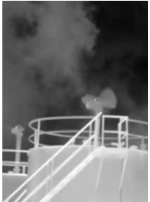
Figure 1: Unmonitored methane leaks discovered by NGO Earthworks in Mexico by using infrared cameras.
